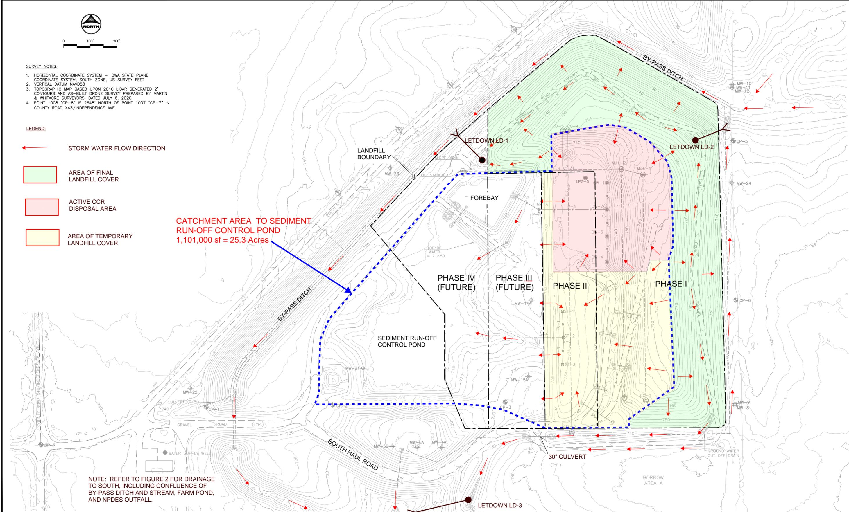
**NOTE: REFER TO FIGURE 2 FOR DRAINAGE TO SOUTH, INCLUDING CONFLUENCE OF BY-PASS DITCH AND STREAM, FARM POND, AND NPDES OUTFALL.**
