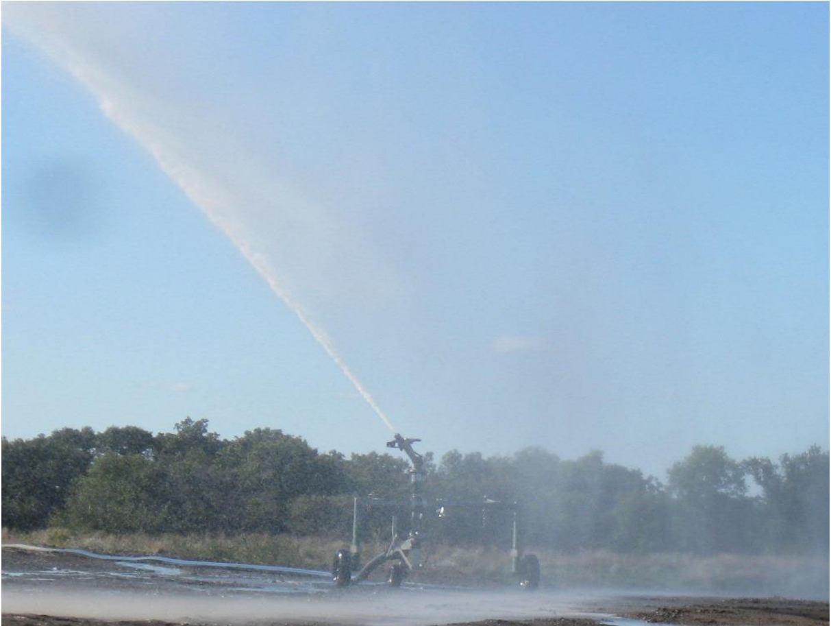
Picture 3: Ag Rain being used to suppress dust on the active area
